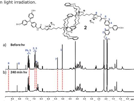
Treatment of the self-assembled structure made of **2** with NaOD led to the reappearance of NMR signals corresponding to the triarylamine core, thus demonstrating the reversibility of the self-assembly upon deprotonation of the rotaxane unit.
