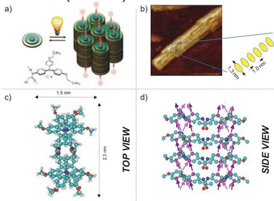
a-b) Visible light irradiation of triarylamine (TAA) solutions produces small amounts of radical cations which trigger the piling up with their neutral counterparts into one-dimensional TAA stacks. These stacks bundle into three-dimensional nanofibers that display metallic conductivity; c-d) Molecular arrangements of TAA in bicolumnar “snowflake” stacks determined by all-atomic modelling (conducting pathways are marked with violet arrows).
