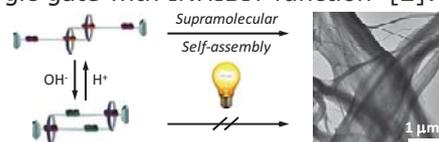
A logic gate based on a bistable [c2] daisy chain rotaxane decorated with lateral triarylamine units is described, giving rise to an INHIBIT logic function using proton concentration and light as inputs, and producing dual color change and supramolecular self-assembly as outputs.
