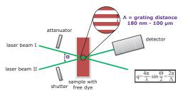
Schematic illustration of the FRS experiment. Through the superposition of two laser beams a holographic grating is created. Depending on the angle  $\theta$  between the beams I and II, the grating distance  $\Lambda$  can be adjusted.
