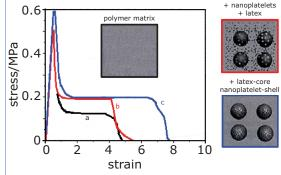
Stress-strain curves for coatings from a) pure polymer, b) pure polymer with nano-platelets and latex, c) pure polymer with latex-core nano-platelet-shell particles.  $^{[3]}$
